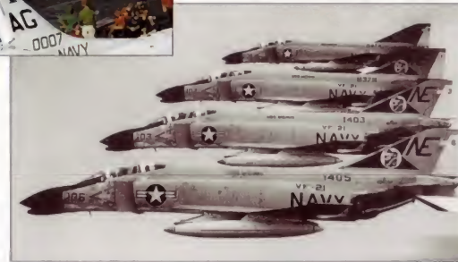
Below: This quartet of F-4Bs, belonging to VF-21 'Freelancers', is shown posing for the camera. The wing fuel tanks are unusual.
